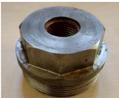
1/2" female NPT-2"male NPT. Stainless steel.
